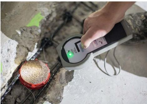
Not visible from the outside: The wireless and energy-less sensor technology is read annually.
