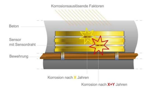
This is how the CorroDec®2G works: direct connection to the top reinforcement layer with corrosion sensors in two levels.
